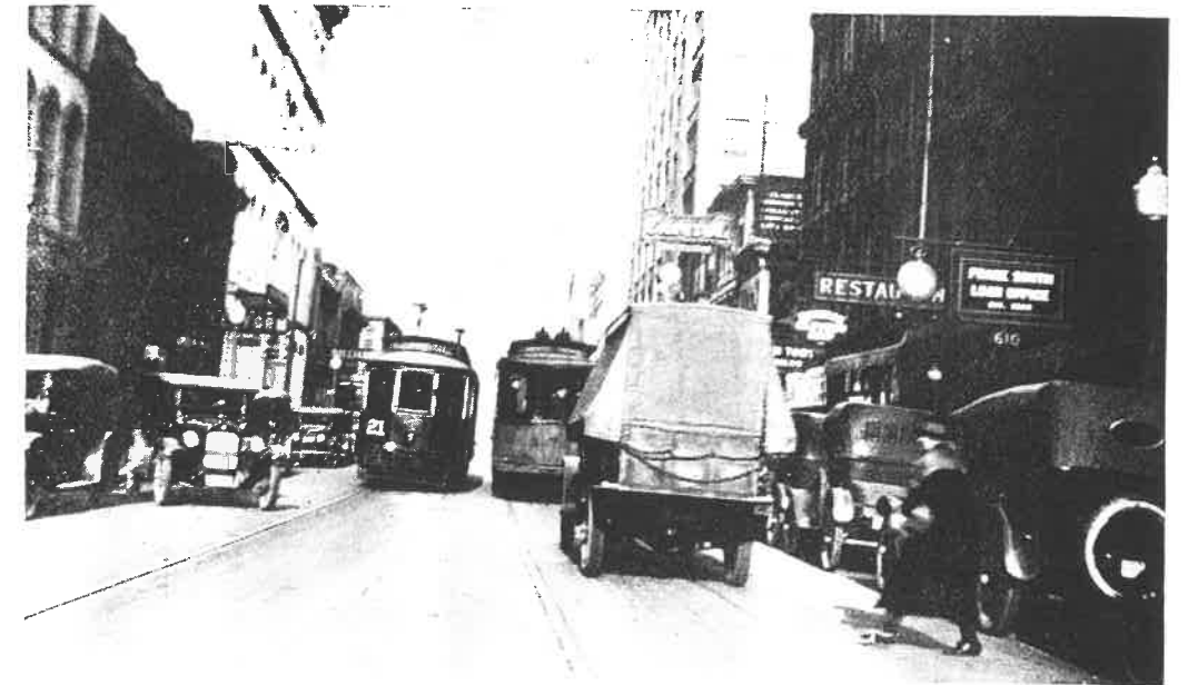
TYPICAL TWO CAR TRACK DOWNTOWN CINCINNATI STREET Stopping street car blocks traffic
