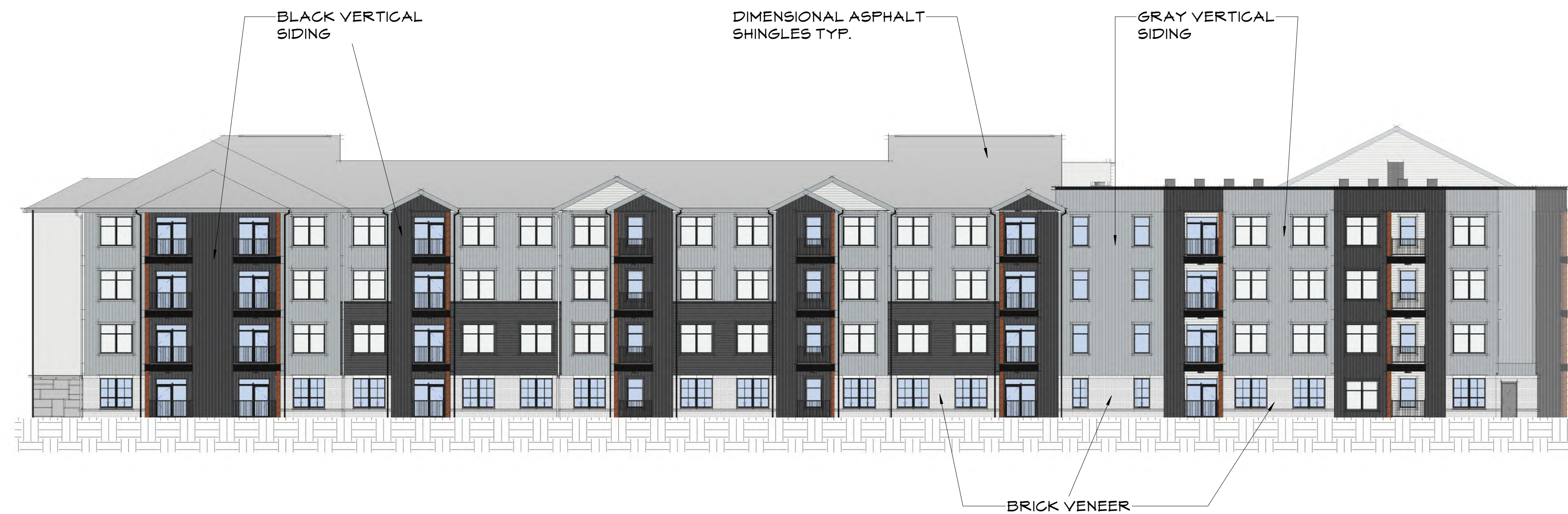
BUILDING 2 NORTH WEST ELEVATION
