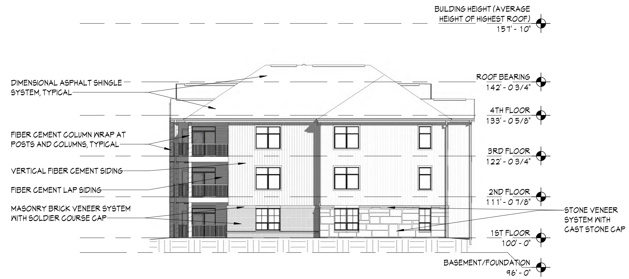
BUILDING 1 WEST ELEVATION 1/16" = 1'-0"
