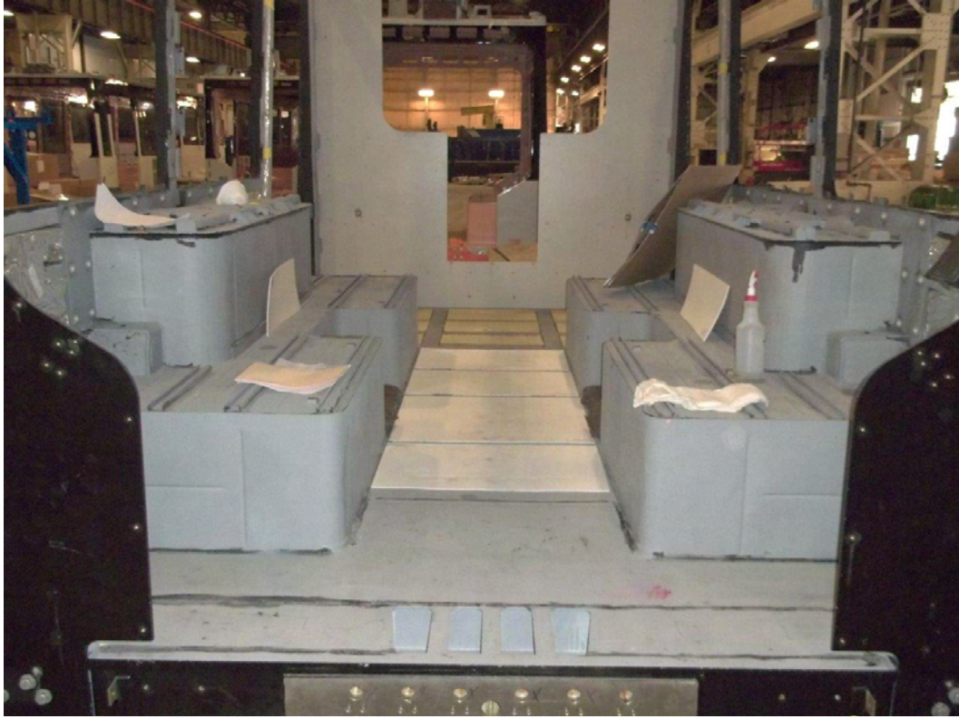
Photo 29: Flooring material installed in car body
