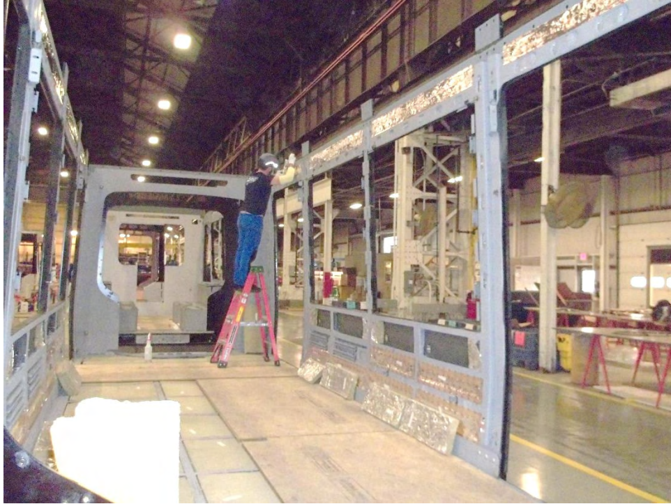
Photo 27: Insulating side panels of car shell
